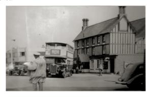
The bus is one of the open staircase AEC Renown six-wheelers of the LT class which were on this route until almost their final withdrawal in the late 1940s. These vehicles were based at Loughton (L) and Leyton (T) garages.
